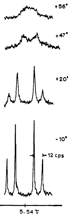
Figure 1. Temperature dependence of the nmr spectrum of the methylene protons of the \alpha -bromopinacolone-boron tribromide complex.
